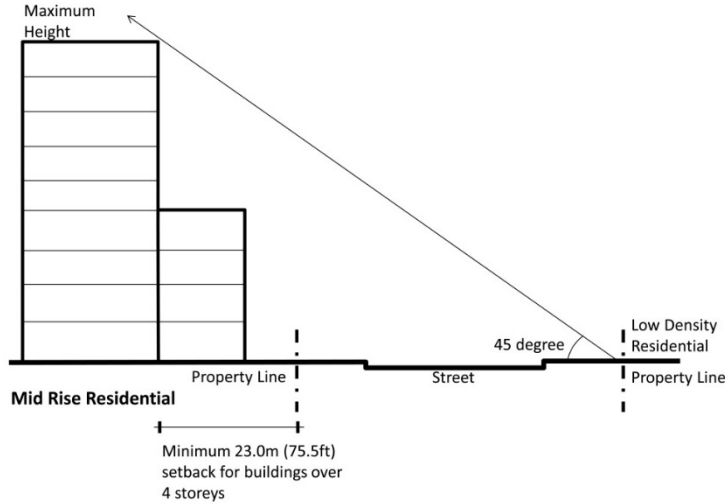
Figure 13.12b: Application of 45 Degree Angular Plane
