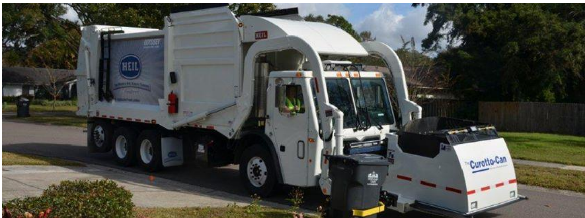
Figure 5.3 Heil Odyssey AFL with integrated Curotto-Can
