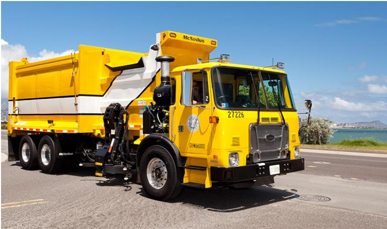
Figure 5.7 McNeilus auto reach automated side loader
