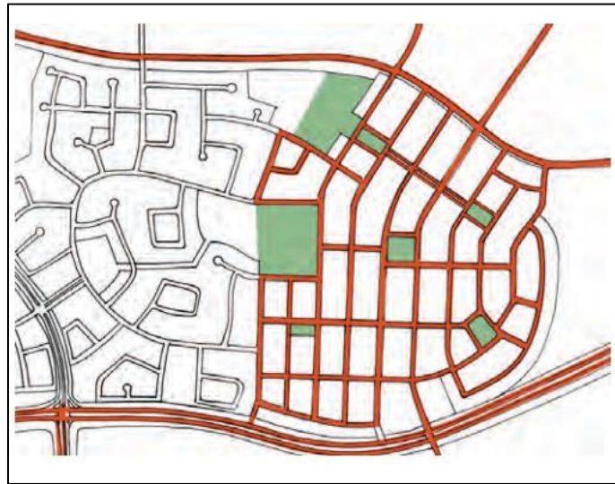
Figure 4. Example of a modified grid pattern (red) compared to a curvilinear loop pattern.
